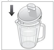
3 Place the glass jug I on the base unit E. Turn the swivel head D clockwise and press to lock securely. Insert the fruit or vegetables in small pieces from the filler spout on the juice extractor lid L and insert pusher O.
